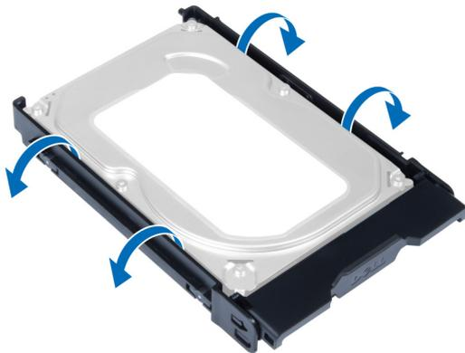
8. Lift the hard drive in an upward direction to remove it from the hard drive bracket.
