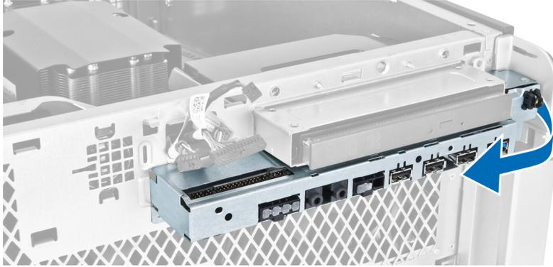
6. Slide the opposite edge of the front I/O panel outward to disengage the I/O module from the chassis.
