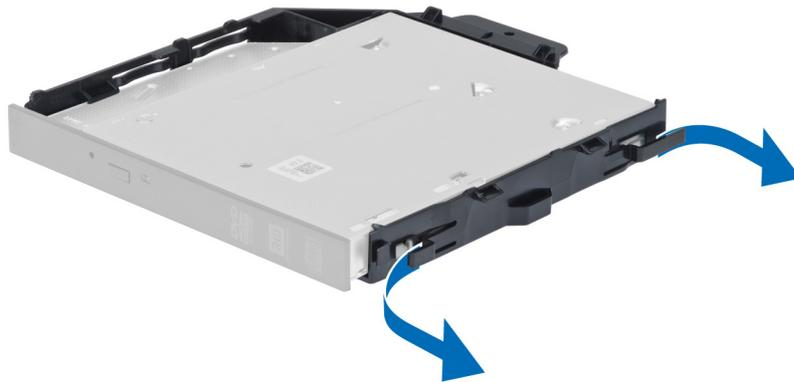
8. Lift the optical drive and remove it from the bracket.
