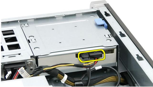
4. Press the release latch (1) and slide the optical drive outward to release it from the drive bay (2).
